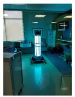
**Ultraviolet germicidal irradiation** (UVGI) is a disinfection method that uses short-wavelength **ultraviolet** (**UV**-C) light to kill or inactivate microorganisms by destroying nucleic acids and disrupting their DNA, leaving them unable to perform vital cellular functions.
